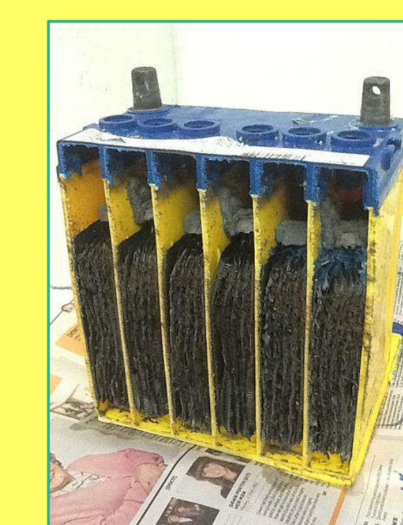
Cut-away view of lead acid battery
